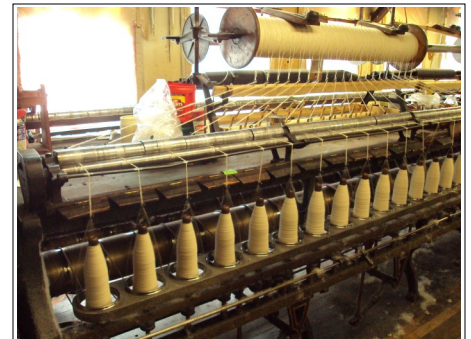
Twister, making two-ply yarn.
